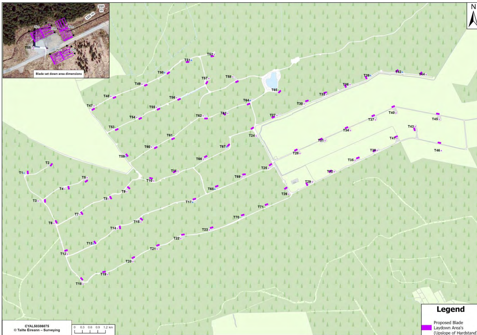
DMP 11 Locations for temporary blade storage areas at each turbine
